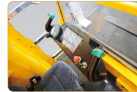
With comfortable seat and adjustable panel. Front panoramic window made of safety glass for protection and a clear view of front forks.
