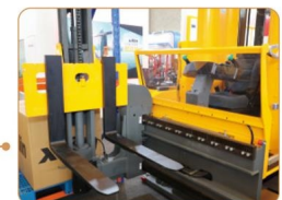
Fork carriage can rotate 180 degrees, flexible for operation in high racking with small aisle.
