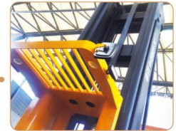
Overhead guard with fans and working light.
