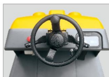
Adjustable steering column with electric F/R lever.
